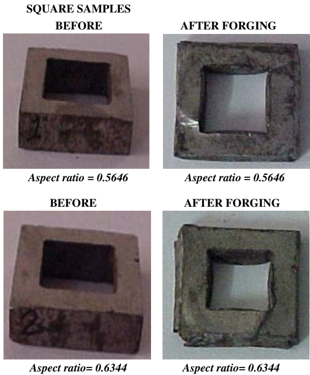
Fig. 2 Square samples of aspect ratio 0.5646 and 0.6344 before and after forging
