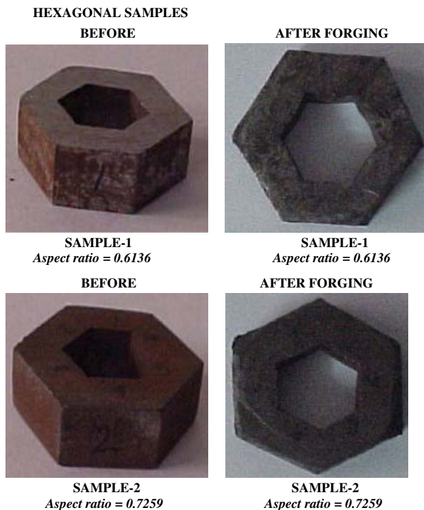
Fig. 4 Hexagonal samples of aspect ratio 0.6136 and 0.7259 before and after forging
