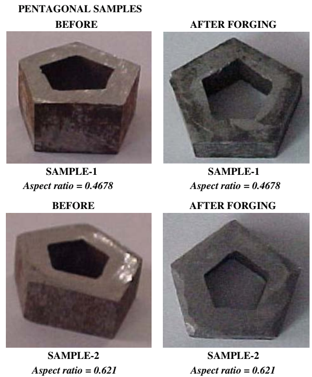
Fig. 3 Pentagonal samples of aspect ratio 0.4678 and 0.621 before and after forging
